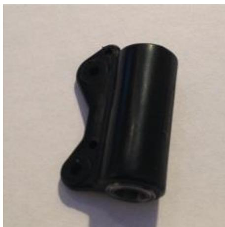
Gooseneck fitting with bearings inserted
