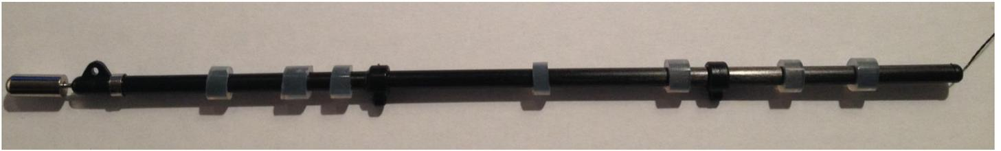
Completed Jib boom kit including silicon rings and 30lb jib leach line
